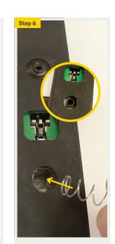
Insert compression spring into Internal body handle hole.
