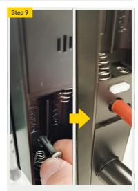
Using a screwdriver and mounting screws, fix the Internal and External bodies together.
