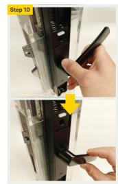
Test lever functionality by lifting and lowering the internal handle. Lifting the internal handle should engage multipoint locking. Lowering the handle should retract multipoint locking.
