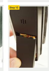
Insert four AA batteries (two in the top and two in the bottom).
