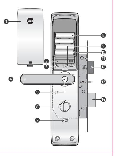
**4. Internal Body** (Internal Body, installation on the inside of the door)
